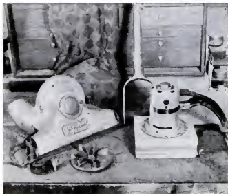
What's left of vacuum cleaner after sander has been built is shown at left. Only parts of vacuum you need are motor and belt pulley.
